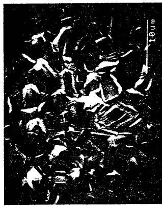
Fig. 5. Scanning electron micrographs of the surface of the scale formed on pure Ni coupons after oxidation in 1 atm O 2 at 1000°C for 24 h: (a, top left) Uncoated Ni; (b, above) Ni/100 Å Ca; (c, left) Ni/250 Å Ca.
